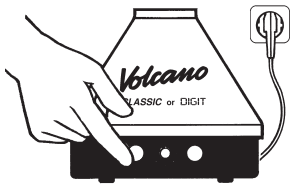
1. Switch heat on (takes 3-5 min.)
